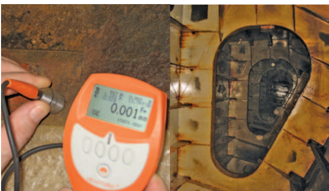
Step test for rust and scale removal (left) Cured treatment on existing paint
